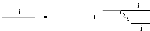
FIG. 4. The diagrammatic analog of Fig. 2 under the mean-field approximation—the two-cell distribution is expressed as the product of two one-cell distributions. Iteration of this equation yields an infinite set of tree-level diagrams.
